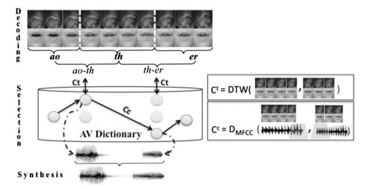
Fig. 9. Phonetic decoding, unit selection algorithm and unit concatenation.
