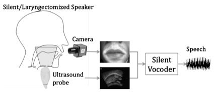
Fig. 1. Ultrasound-based silent speech interface (schematic).
