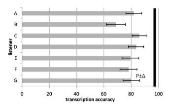
Fig. 10. Evaluation of the synthesized speech intelligibility when the phonetic prediction is correct (transcription accuracy and confidence interval). The black vertical bar indicates the average transcription accuracy of the original sentences (97%).
