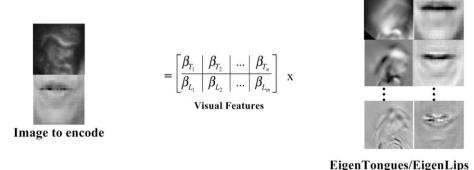
Fig. 5. Encoding ultrasound and optical images of the tongue and lips using the EigenTongue/EigenLips decomposition.
