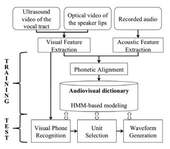
Fig. 2. Overview of the segmental vocoder.
